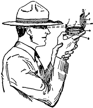
FIGURE 56.—Prismatic compass, showing compass open and in position for measuring azimuth in daylight.
