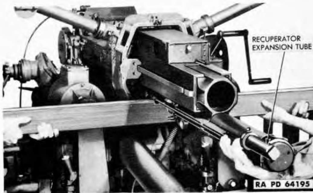
Figure 67 – Sliding Gun From Cradle
