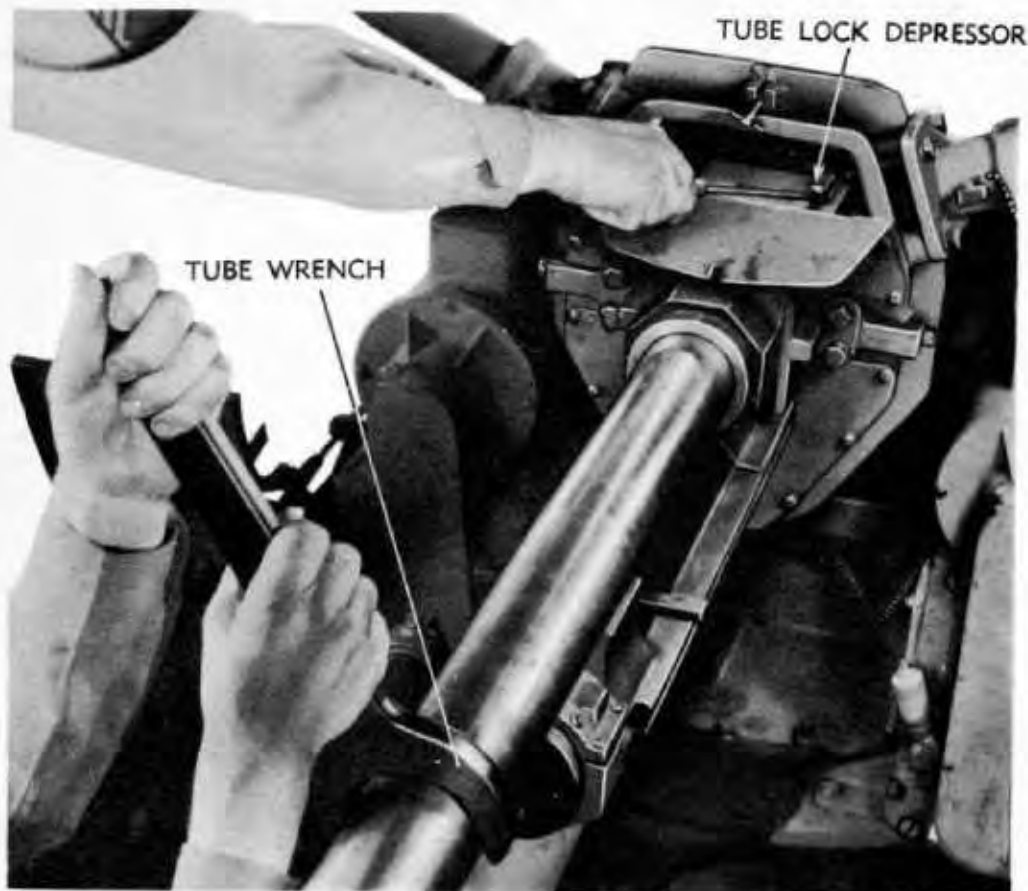
Figure 61 – Loosening Gun Tube
