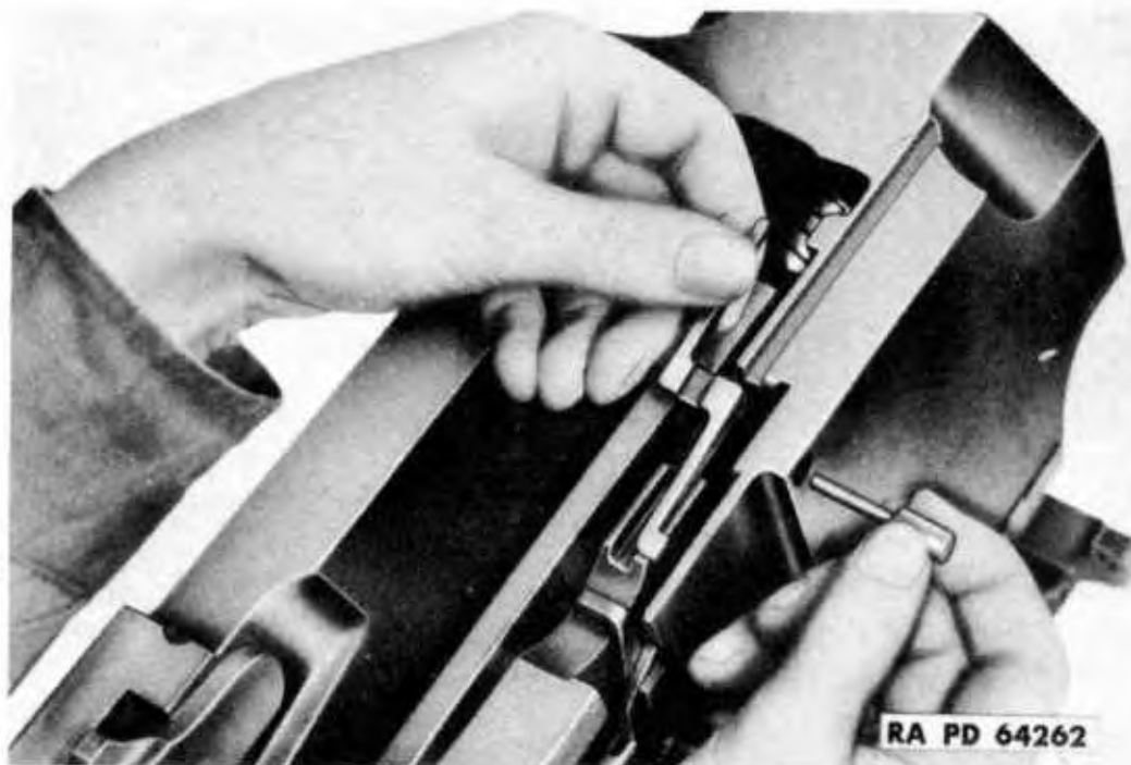
Figure 98 — Removing Trigger Trip
