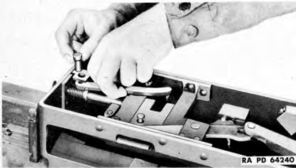
Figure 107 — Removing Feed Slide Return Lever
