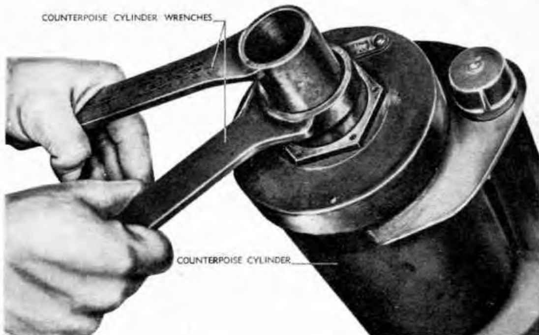
Figure 138 — Adjustment of Counterpoise Spring
