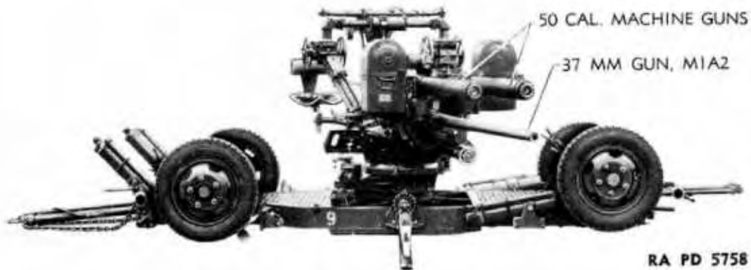
Figure 2 — 37-mm AA Gun Carriage M3E1
