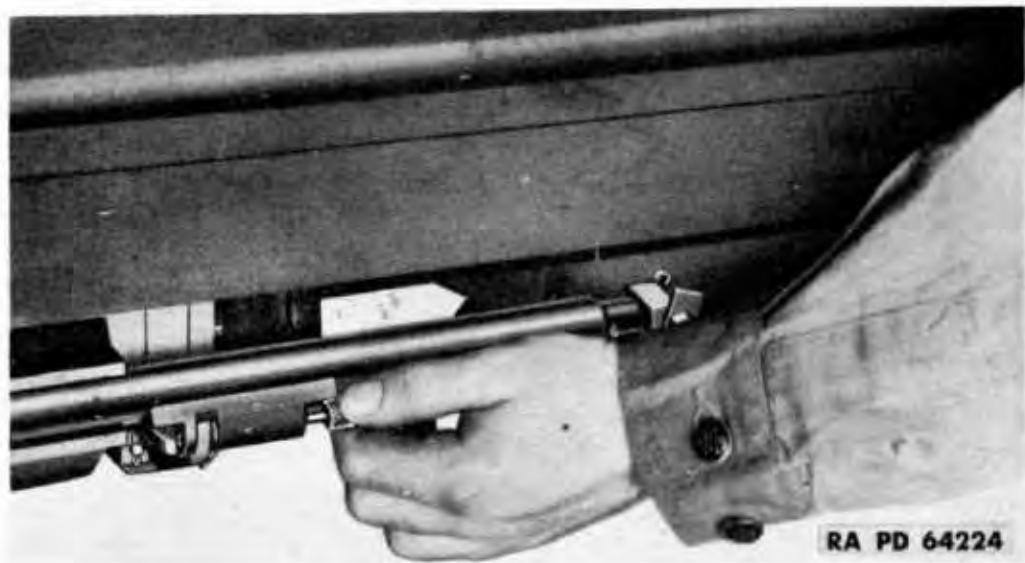
Figure 81 – Disconnecting Driving Spring Tube
