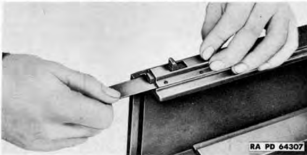
Figure 123 – Installing Back Plate Latch Assembly
