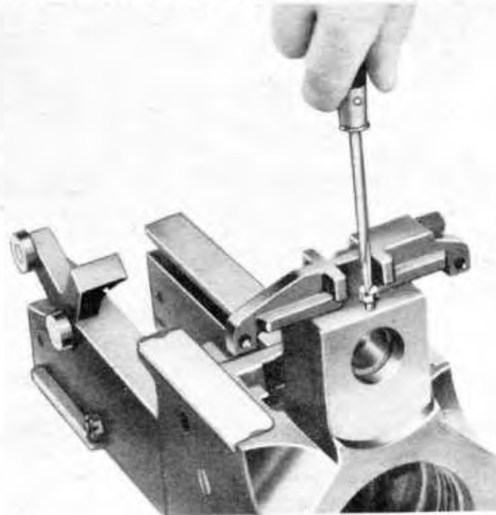
Figure 93 — Removing Breechblock Stop Pin and Stop
