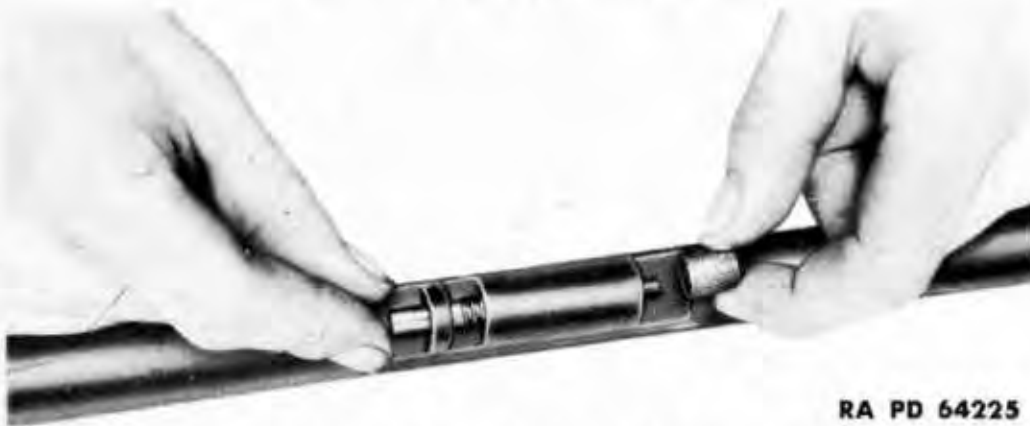
Figure 82 — Removing Driving Spring Tube Connection Pin Knob
