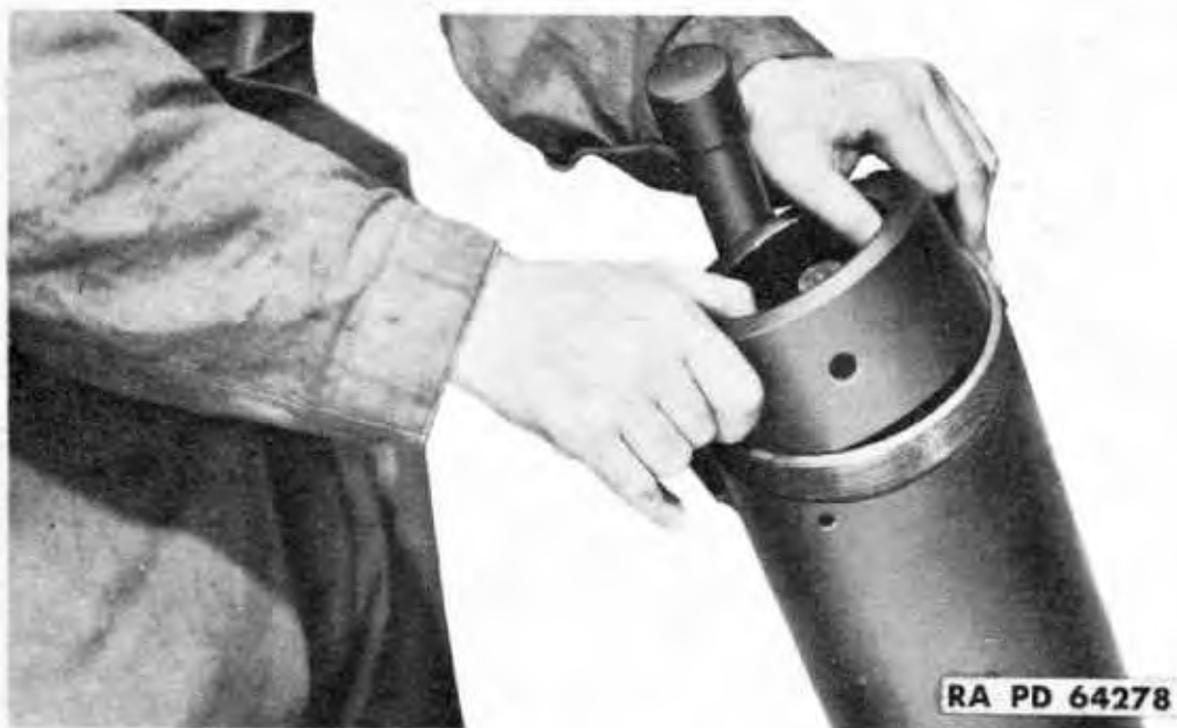
Figure 130 — Placing Spring Compressor Spacing Collar in Cylinder
