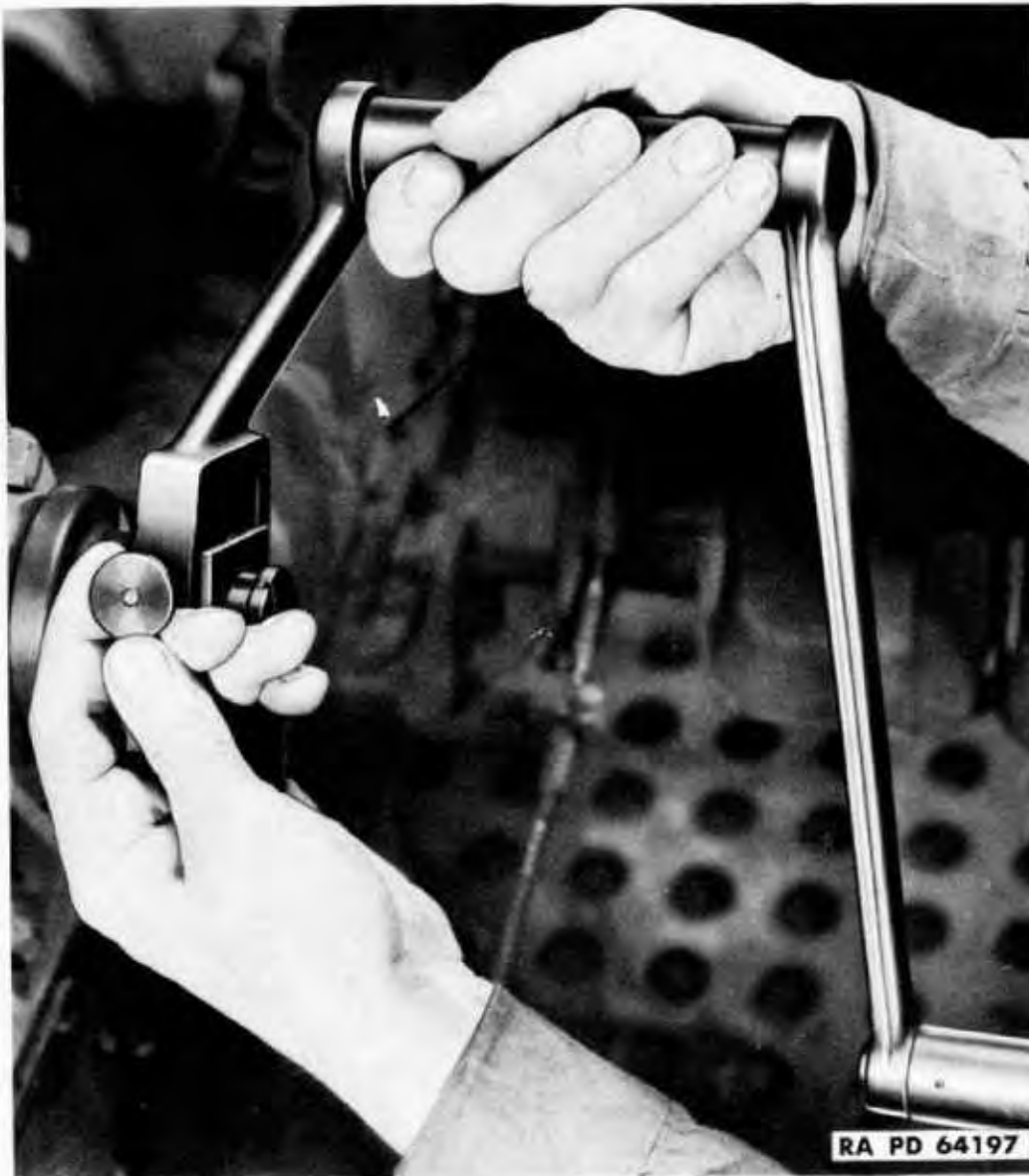
Figure 49 — Removing Hand Crank
