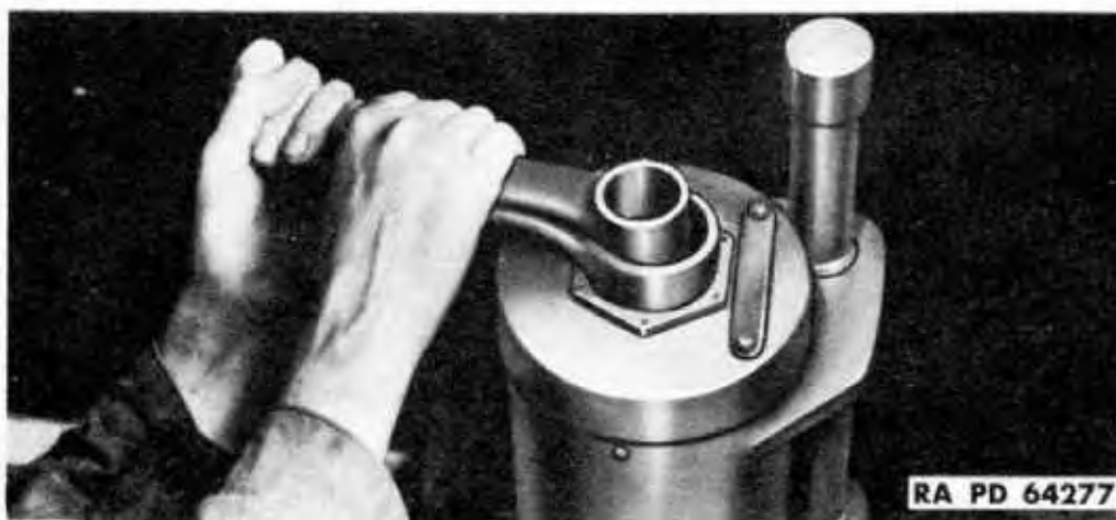
Figure 131 — Removing Counterpoise Rod Nuts
