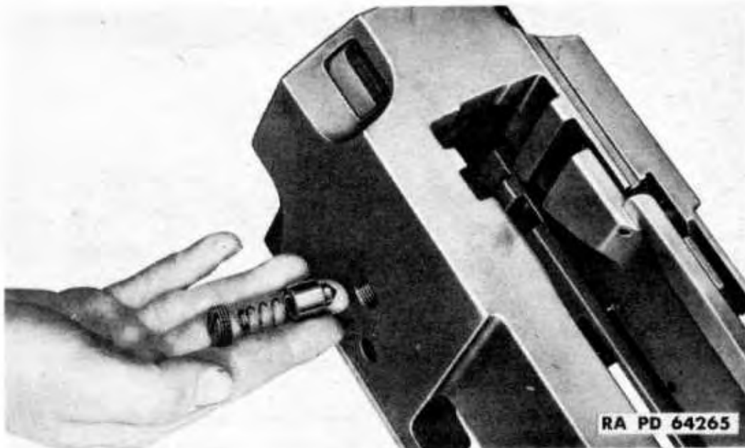
Figure 102 – Removing Breechblock Plunger
