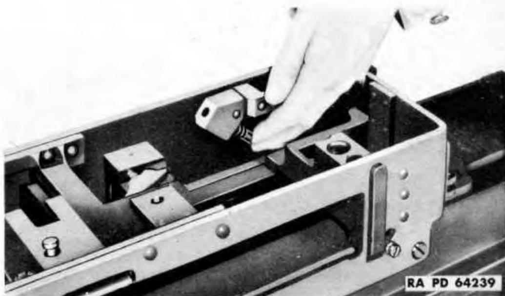
Figure 110 — Removing Feed Lever Spring Plunger and Springs
