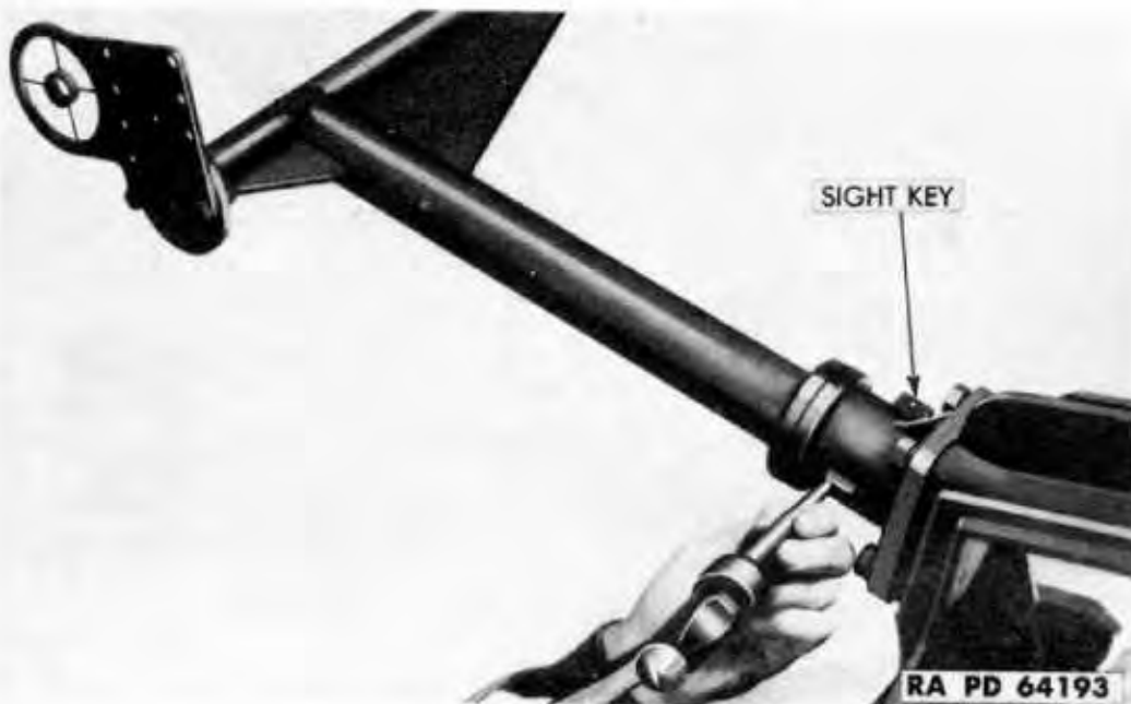
Figure 125 — Removing Sight Key
