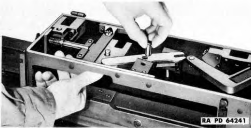
Figure 108 — Removing Feed Slide Lever
