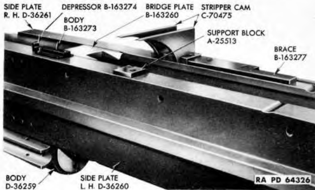
Figure 120 — Trunnion Block Subassemblies
